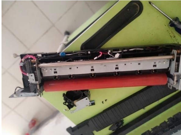
Thatta Photocopier Machine Pressure Roller and Sensor Repaired
