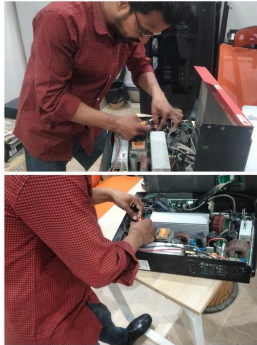
Solar Inverter Fault Diagnose and Cooling Fan changed
